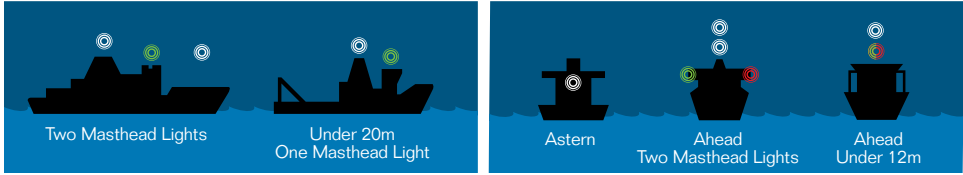
Figure 9-1 Power driven vessels – Examples
