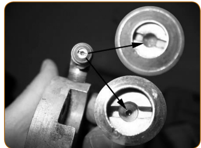
Photo 4: Return-to-tank bleed orifice (shown frozen and thawed for comparison)
