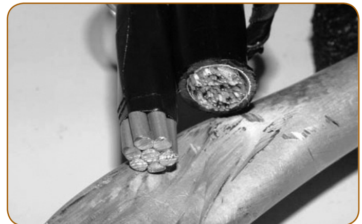
Photo 2: Cable markings on crankcase vent tube
