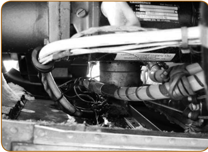
Photo 1: Fuel distributor valve installation in the lower front engine area
