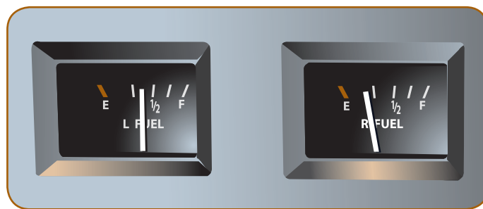
A common factor in fuel starvation incidents: fuel gauges that do not indicate properly
