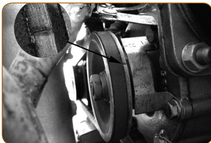
Photo 2: Correct timing mark
