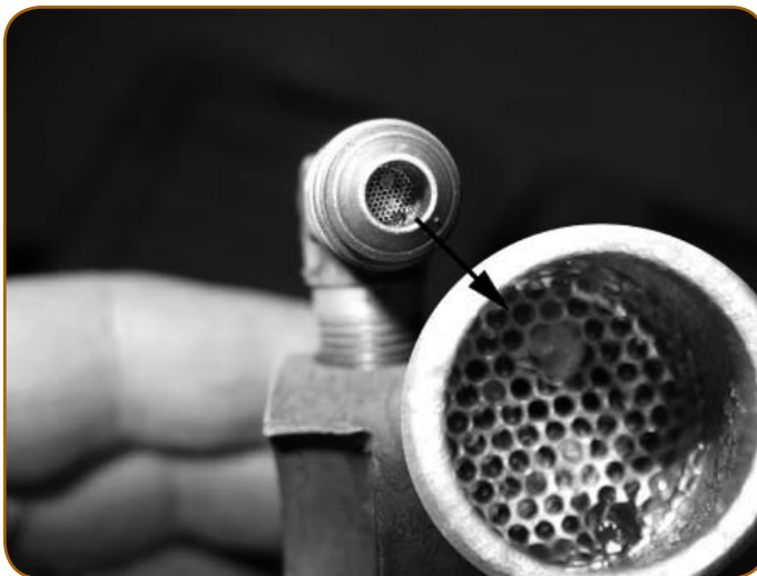
Photo 3: Super-cooled droplet ice formation on the servo bleed screen
