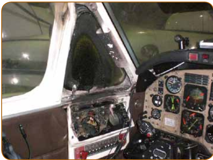
Damage caused by fire in the cockpit of a King Air 100.
