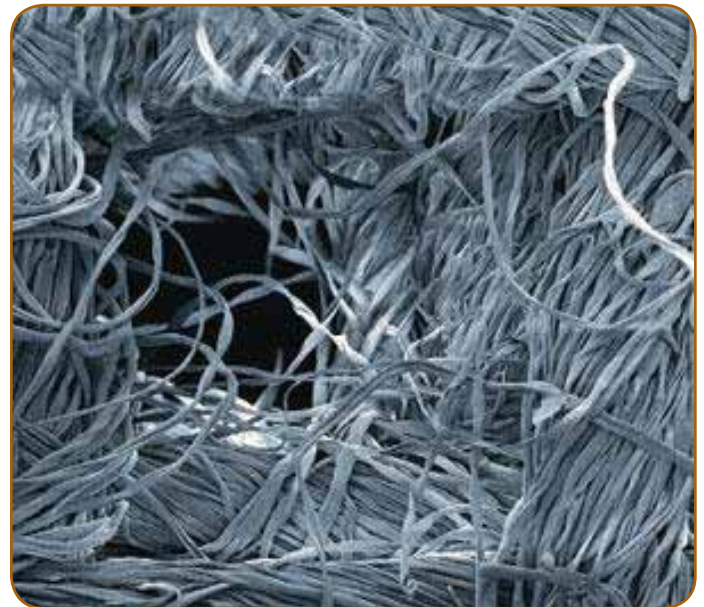
Wet media, as its name implies, is a type of media that requires a tacky oil to be applied to a substrate to act as the dust trapping agents.
