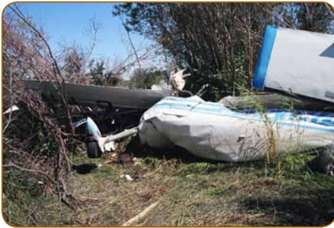
This 2006 crash was a case of mishandling of the aircraft, resulting in an aerodynamic stall, followed by a spin.
