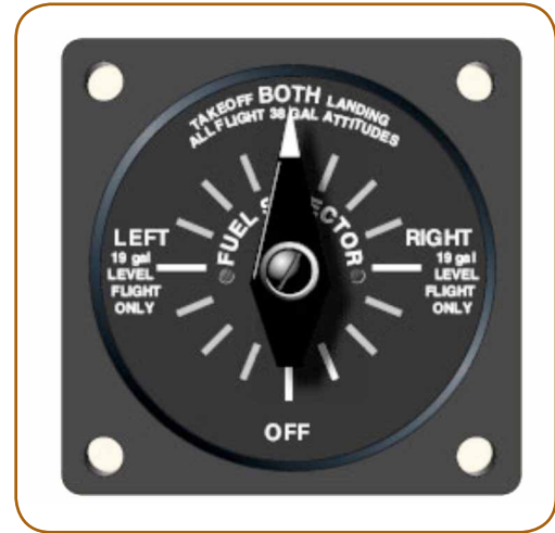
There is no ON position on this valve; only BOTH, RIGHT, OFF, and LEFT.
