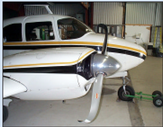
Propellers are shown after the occurrence, damaged beyond repair.
