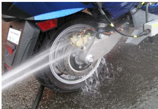
Figure 9 – Vectrix brakes being soaked in water
