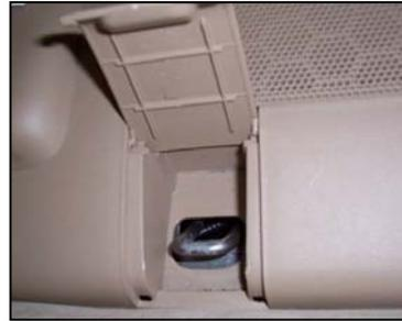
**Figure 6. Top tether anchor indicator symbol (car).**
