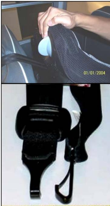
**Figure 3. Top tether and lower attachments on CRS C.**
