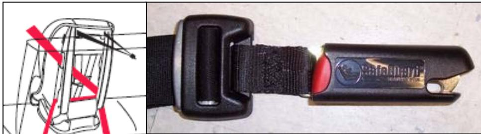
**Figure 2. Top tether and lower attachments on CRS B.**
