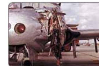
Bird strike damage due to Turkey Vulture
