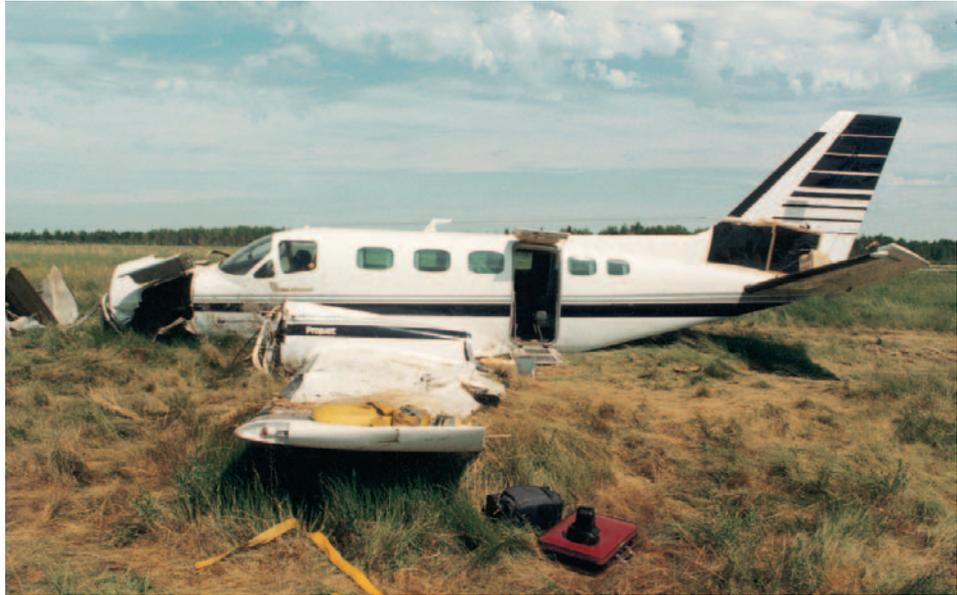
**Plate 3** This accident involving a Cessna 441 Conquest at Fort Frances, Ontario, was the result of a gull being ingested in the intake of the #1 turboprop engine.
