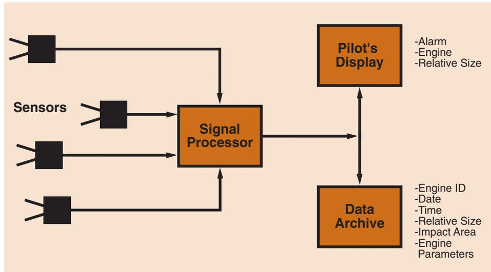
**Figure 14.2** Outputs from the FOIDS Signal Processor
