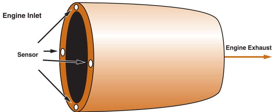
**Figure 14.1** Foreign Object Ingestion Detection System (FOIDS)
