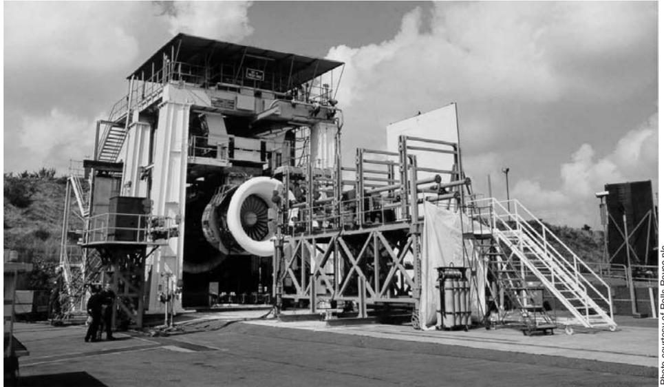
**Figure 12.2** Bird impact test facility for jet engines.
