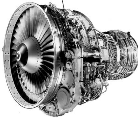
Figure 5.4 CFM56 Turbofan Jet Engine
