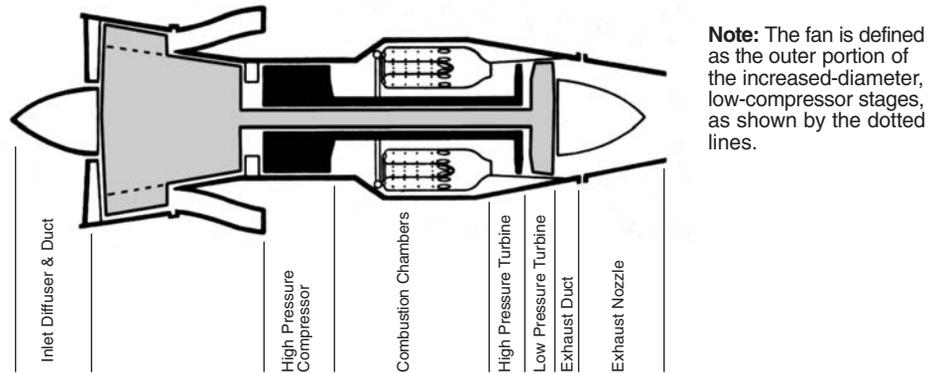
**Figure 5.7** Schematic of a Turbofan Engine
