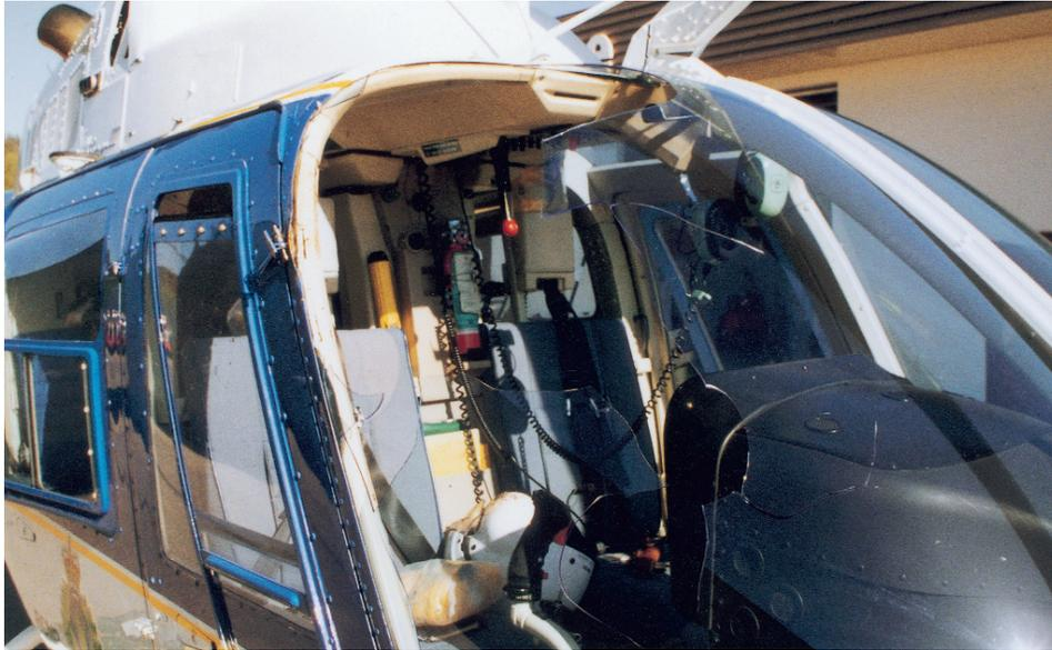
**Plate 5** An impact with a Western Grebe (3 lbs) caused considerable damage to this helicopter. The bird struck the pilot in the face. (See plates 6 and 7)
