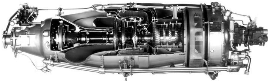
Figure 5.6 Cutaway of a Turboprop Engine
