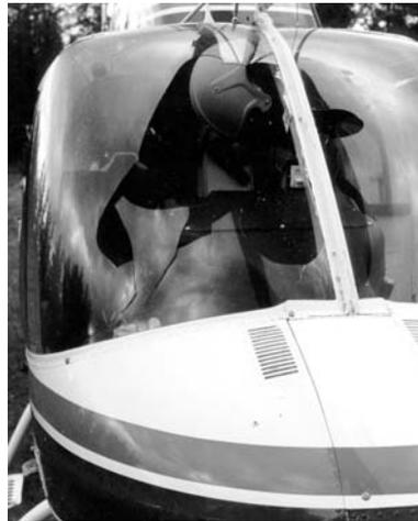
Helicopters operate in environments in which they are highly vulnerable to windshield damage from bird impacts.
